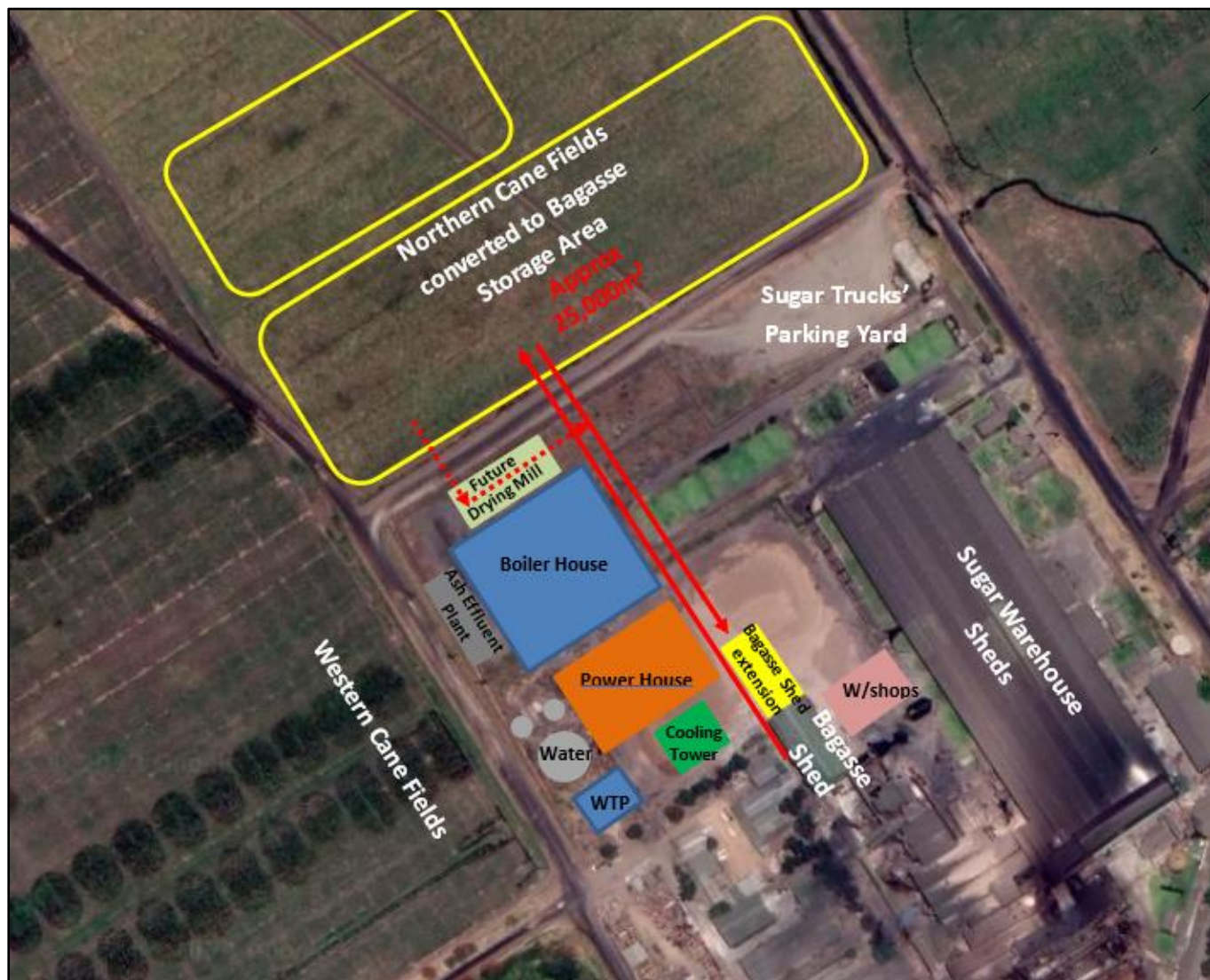
FIGURE 2-4: PROPOSED PRELIMINARY LAYOUT OF THE COGENERATION POWER PLANT (AT DESKTOP LEVEL)
